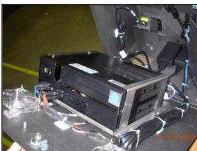
The LobbyGuard Kiosk runs on a slim-line integrated PC running the Windows Operating System. All peripherals for the kiosk are attached to USB ports on the PC. The kiosk ships with a USB mouse and keyboard for use by administrators when needed. The kiosk is designed to be maintenance free and easy to use.
